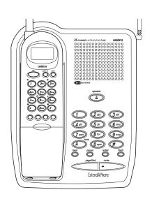
2. Make sure the Battery icon lights. If the icon doesn't light, check to see that the AC adapter is plugged in, and that the Handset is making good contact with the Base Unit charging contacts.
